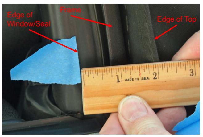
Fabric of top is almost two inches too short. This causes water Intrusion. Top should cover the frame and overlap window/seal.
