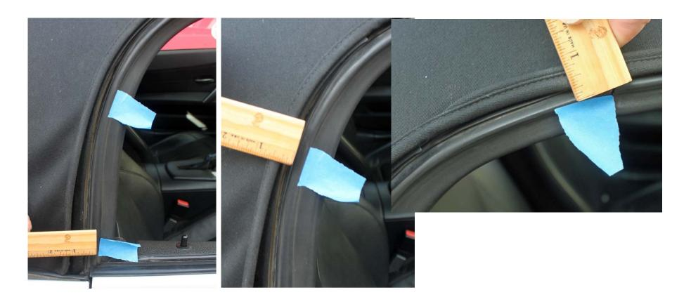
Passenger side window finish was not as bad as driver side but will not prevent water intrusion by passing the window/seal and infiltrating around the uncovered frame
